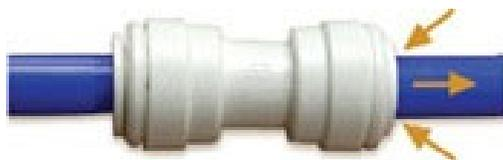
Push in the collet and remove tube. To disconnect, ensure the system is depressurized before removing tube. Push in collet squarely against face of fitting. With the collet held in this position, the tube can be removed.
