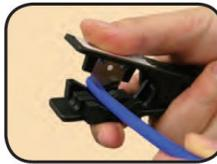
Cut the tube square. It is essential that the outside diameter be free of score marks and that burrs and sharp edges be removed before inserting into fitting. For soft, thin-walled tubing we recommend the use of a tube insert.
